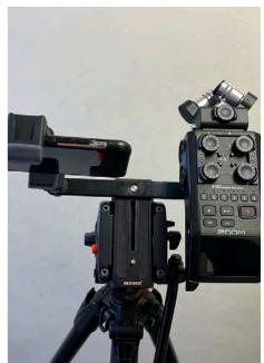
Then simply position the mic stand (with phone and H6 attached) open your camera and record a video as normal. To listen to the video you can plug the headphones into the H6, any audio played on the phone will come out through headphones via the H6.
